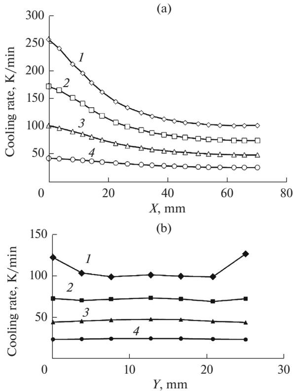
**Fig. 3.** Change in the cooling rate of the melt in transverse section of the plate along  $X_0$  (a) and  $Y_0$  (b) at chill mold temperatures: (1) 200; (2) 300; (3) 400; (4) 500°C.
