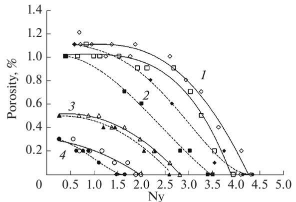
**Fig. 5.** Volume fraction of pores depending on the value of the Niyama criterion during casting of the given plate into chill mold at temperatures: (1) 200; (2) 300; (3) 400; (4) 500°C. Solid lines—for nodes along the line  $X_0$ ; dashed lines—for nodes along the line  $Y_0$ .
