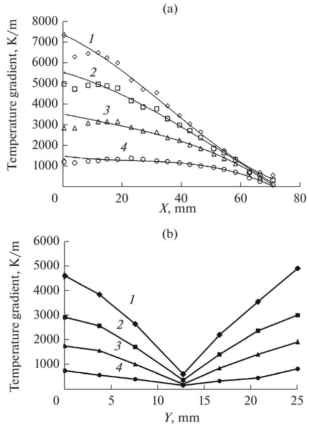
Fig. 2. Change in the temperature gradient in transverse section of the plate along  $X_0$  (a) and  $Y_0$  (b) at chill mold temperature: (1) 200; (2) 300; (3) 400; (4) 500°C.
