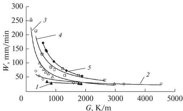
**Fig. 6.** Lines of constant porosity depending on the temperature gradient and crystallization rate: (1)  $P = 0.1$ ; (2) 0.2; (3) 0.5; (4) 1.01; (5) 1.1%.
