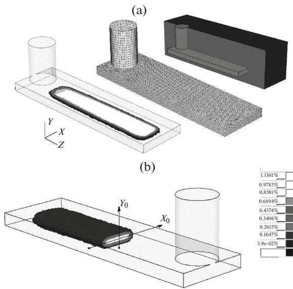
**Fig. 1.** Appearance of casting and chill mold, finite-element model of the casting and porosity in the central (a) and transverse (b) sections of the plate. Central lines  $X_0$  and  $Y_0$  start on the surface of the casting.
