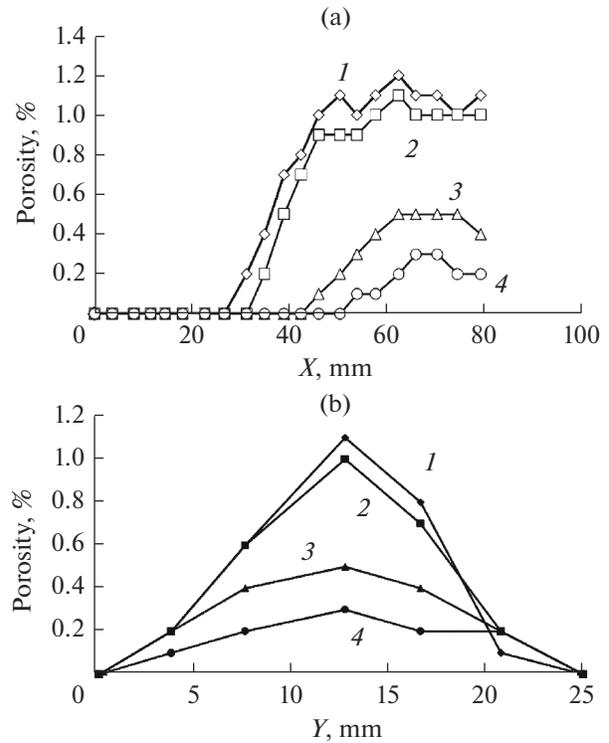
**Fig. 4.** Computed volume fraction of pores in transverse section of the plate along  $X_0$  (a) and  $Y_0$  (b) at chill mold temperatures: (1) 200; (2) 300; (3) 400; (4) 500°C.
